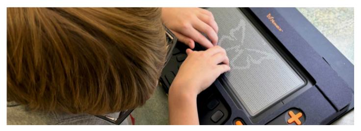
A client uses the Monarch digital Braille reading device.
